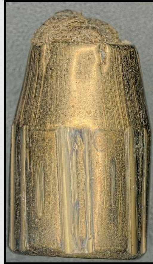
Figure 7 Striations on the surface of a fired bullet
